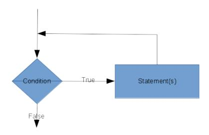
Figure 1: While loop flowchart
